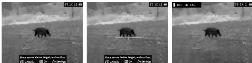
FIGURE 2-10. DISTANCE MEASUREMENT
