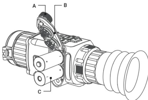
FIGURE 2-1. BATTERY INSTALLATION
