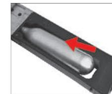
Activate the CO<sub>2</sub> cartridge by turning the screw clockwise, intentionally puncturing the cartridge.
