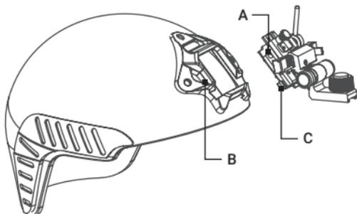
FIGURE 2-10. HELMET MOUNT G50S FOR SHROUD
