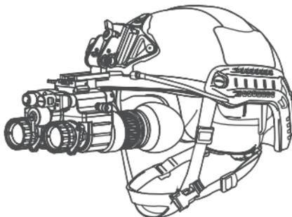
FIGURE 2-5. DOVETAIL TYPE HELMET MOUNT
