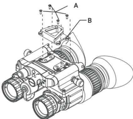
FIGURE 2-4. INSTALLING A MOUNTING BRACKET
