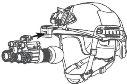
**FIGURE 2-6. BAYONET/HORN TYPE HELMET MOUNT**
