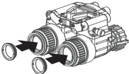
FIGURE 2-13. DEMIST SHIELD INSTALLATION
