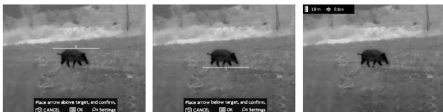
FIGURE 2-13. DISTANCE MEASUREMENT
