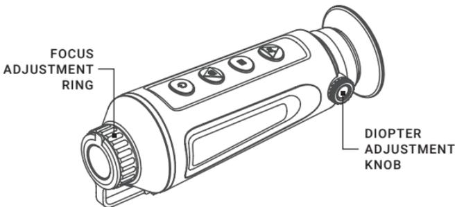
FIGURE 2-4. DIOPTER AND FOCUS ADJUSTMENT
