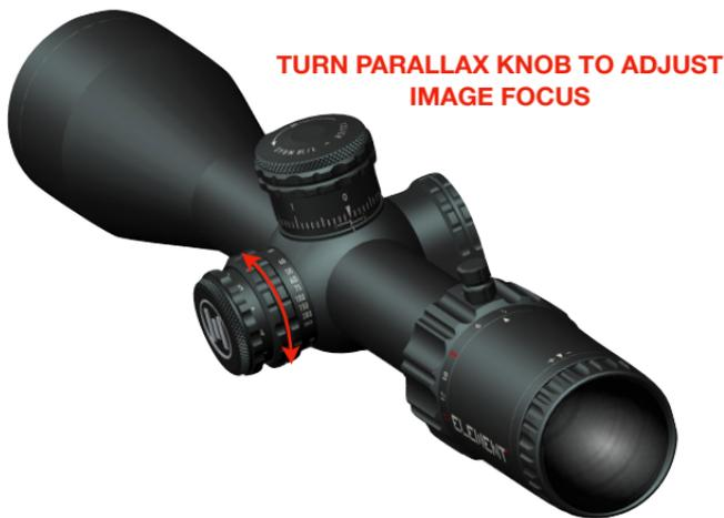
**Tip:** Place your riflescope in a fixed position and change the position of your eye (up/down, left/right) while adjusting parallax. If parallax is not set correctly, there will be apparent movement of the reticle in relation to the target. Adjust the parallax until this movement is eliminated.
