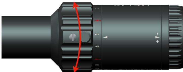
This model is in Second Focal Plane, which means that the subtensions of the reticle will change with respect to the target as magnification is changed – The reticle is calibrated at 16x, and reticle subtensions will be correct at this setting.
