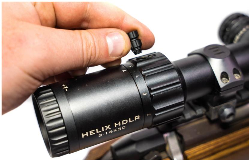
Your HELIX HDLR will need to be zeroed after it has been fitted to your rifle. The Elevation & Windage turrets feature different designs, and need to be reset differently. The first step is to lift the elevation turret housing and remove the zero stop mechanism to allow a full range of adjustment.
