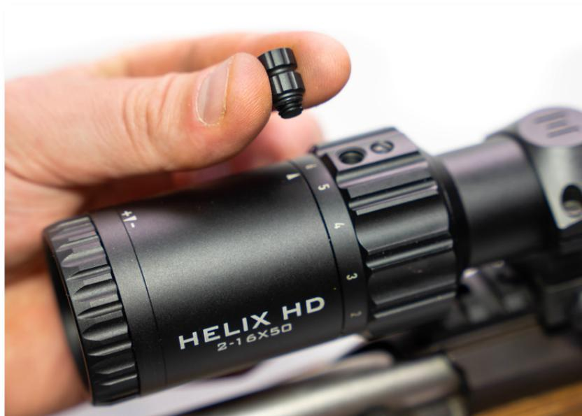
Your HELIX HD will need to be zeroed after it has been fitted to your rifle. The first step is to remove the turret caps to expose the turrets.
