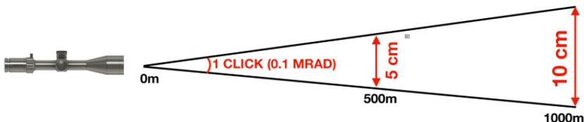
Most rifle scope turrets are divided up into smaller units for more precise adjustments. The HELIX HD features 1/10 MRAD click adjustments, but we have engraved “1 Click = 1 cm @ 100m” to make things easier to understand!
