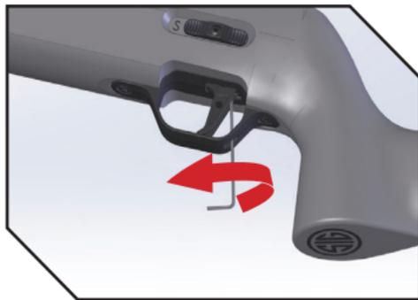
2. To increase the length of the second stage, turn the screw counter-clockwise (outward).
