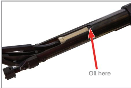
It is also recommended to lubricate the pump arm linkage and bolt pivot points with machine oil every six months.
