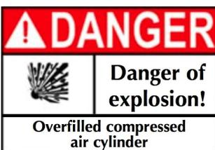
**CAUTION:** USE ONLY DRY, FILTERED COMPRESSED AIR OR NITROGEN IN THE CYLINDER. USE NO OTHER GAS, INCLUDING OXYGEN, WHICH
