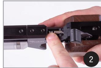
3. Ensure the dry fire switch is in the "F" position. Close the cocking lever by pushing it forward and down, until it returns to the full closed position. This will load the pellet into the barrel. (Fig 3).
