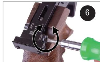
**Elevation Adjustment (Up/Down):** Turn the screw in Figure 7 clockwise to move the rear sight down. Counter-clockwise to move the rear sight up.
