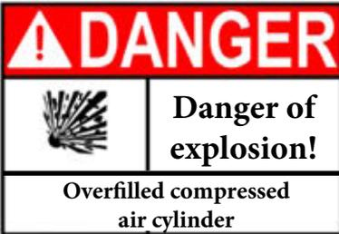
Do NOT exceed maximum fill pressure of 200 bar/3,000 psi at room temperature!
