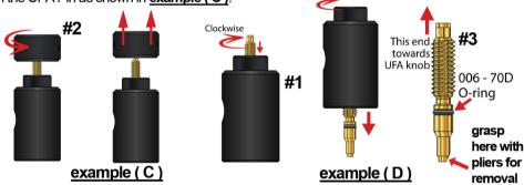
4.To remove the UFA pin (part #3) from the UFA body (part #1) screw the UFA pin CLOCKWISE INTO the UFA body from the top portion of the UFA until the UFA pin comes out of the bottom of the UFA body as shown in example (D).
