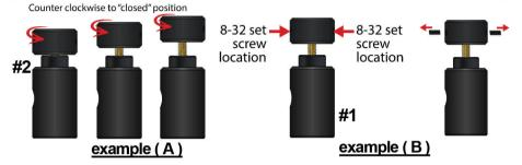
3. To remove the UFA knob ensure the 8-32 set screws are loosened and turn the UFA knob (part #2) counter clockwise towards the "closed" position until the UFA knob is fully removed from the UFA Pin as shown in example (C).
