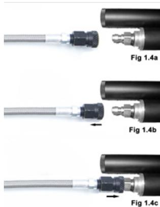
If the collar is hard to move once filling is complete do not force it as pressure may be present. Make sure the hose is fully drained and never remove the qd under any pressure!
