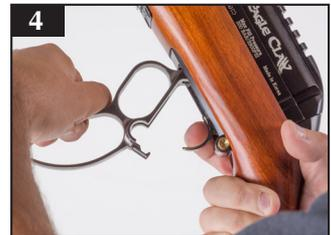
**CAUTION:** HOLD ONTO THE COCKING LEVER TIGHTLY, IT WILL CLOSE RAPIDLY IF YOU SQUEEZE THE TRIGGER WITHOUT HOLDING ONTO IT AND MAY PINCH YOUR FINGERS.
