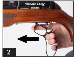
3 - To reload, push the cocking lever forward until it stops, this will cock the hammer and cycle the magazine. (Fig. 2)
