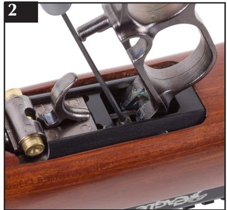
**! WARNING:** THIS ADJUSTMENT AFFECTS SEAR ENGAGEMENT. DO NOT OVER-ADJUST, AS THIS MAY CAUSE THE AIRGUN TO FIRE PREMATURELY OR NOT OPERATE CORRECTLY AND MAKE THE AIRGUN UNSAFE. ALWAYS CHECK YOUR SETTINGS TO ENSURE CORRECT AND SAFE OPERATION OF THE AIRGUN. ALWAYS ENSURE THAT OPERATION OF THE SAFETY IS UNAFFECTED BY ANY ALTERATIONS YOU MAKE TO THE TRIGGER MECHANISM.
