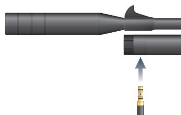
2. Ensure that all components are clean from dirt. Insert the quick-fill adapter into the intake valve and start filling. If you use a scuba tank, fill **slowly** to prevent heat building.
