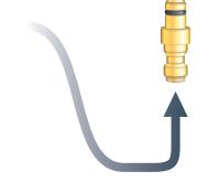
1. Read all instructions about your charging equipment and connect the quick-fill adapter to it. **Please note that your charging equipment must include a pressure gauge (manometer)!**
