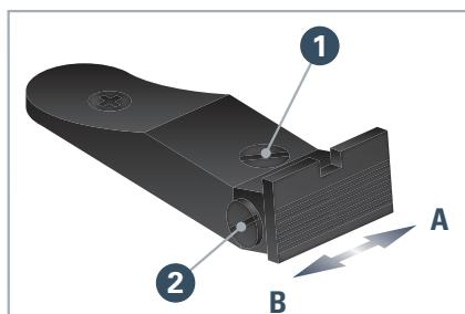
**Elevation adjustment:** If the point of impact is too high: turn screw **1** clockwise. If the point of impact is too low: turn screw **1** counterclockwise.
