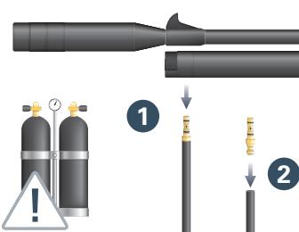
4. **Scuba tank:** BLEED the fill hose COMPLETELY before disconnecting the quick-fill adapter from the air pistol to avoid hose whip and possible injury.
