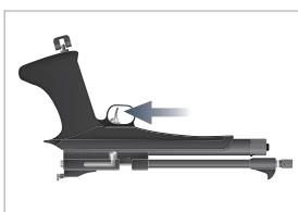
Clean your airgun at regular intervals (500 shots) using a CO<sub>2</sub> maintenance capsule. Remove all pellets from the airgun, insert the CO<sub>2</sub> maintenance capsule and close the CO<sub>2</sub> compartment. Hold the airgun as shown and fire at a safe target until the capsule is empty.
