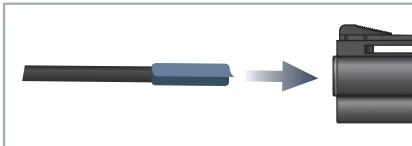
2. Clean the barrel with some gun oil. Insert the rod as shown.
