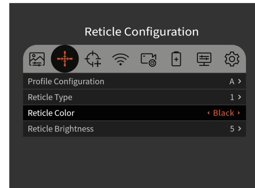
**Reticle BRI:** Reticle BRI can be adjusted within 1-10 levels.
