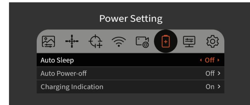
**Auto power-off:** The automatic Power-off time can be set to 15/30/60 minutes. If there is no operation within the set time, the power-off will be activated, and the scope will be powered off.
