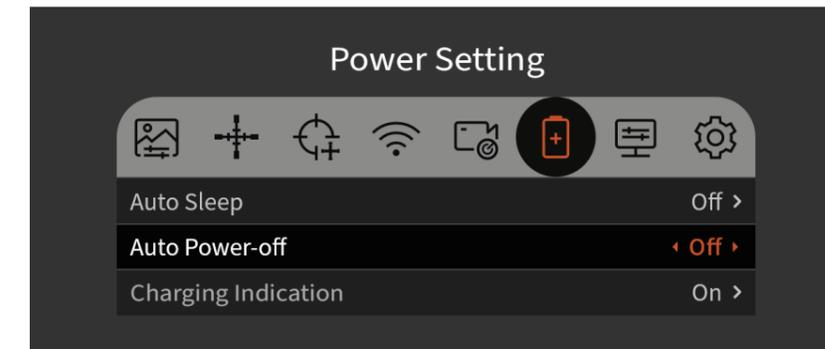
**Charging indication:** Switch that turns On/Off the charging port indication light.
