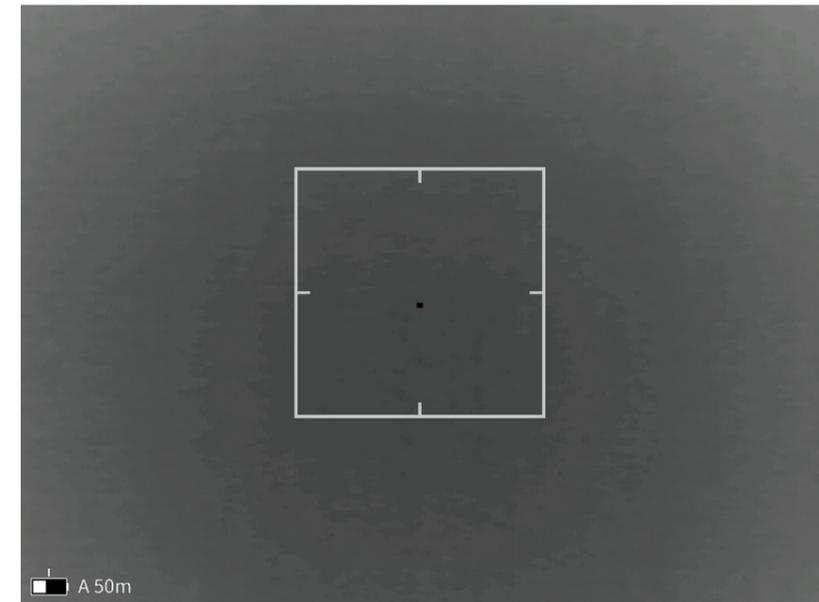
**Videos:** When the scope is turned on and the menu is not activated, long press the "Shutter Button" to start recording, and long press again to end recording. During the recording process, short press the "Photo Button" to take a photo and freeze it for 300ms, and then restore the real-time image.
