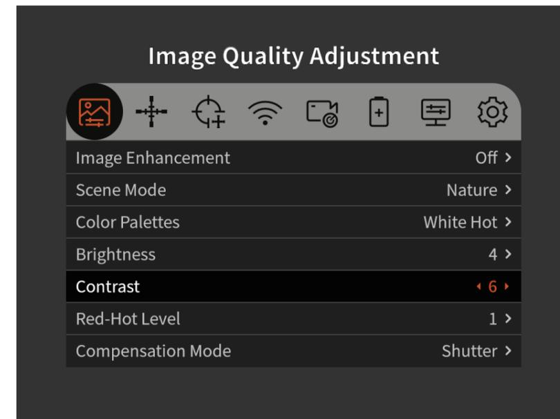
**Brightness:** Detector brightness can be adjusted within 1-10 levels.
