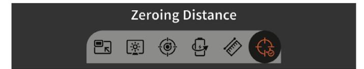
Go to Zeroing Settings interface via the main menu, select the same distance preset by short cut menu to start zeroing in process. Aim the reticle center to the center of the target, and hold the rifle as stable as possible and fire a bullet. Rotate the menu knob to turn on the freeze option
