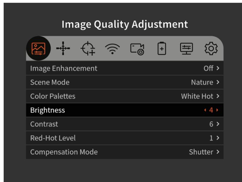
**Red Hot level:** Red hot level can be adjusted within 1-10 levels.
