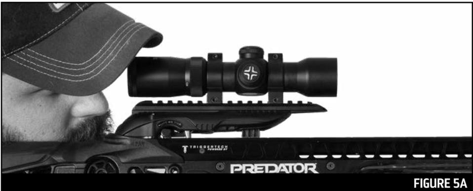
**Assembly Tip:** Ensure the scope rail mounts sit perfectly level on the picatinny scope rail. The adjustable scope ring screws may need to be loosened to ensure the scope rail mounts sit perfectly flat.
