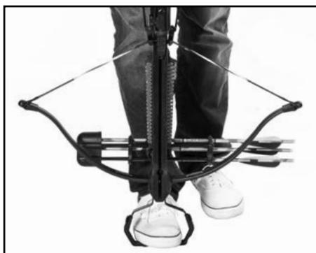
It's essential that you inspect the rope cocking device cord for frays or damage prior to cocking. A frayed or damaged cord may break and result in catastrophic damage to your crossbow and/or may result in serious personal injury. If the rope cocking device shows any signs of wear, DO NOT use it. Contact your local dealer or a Barnett customer service representative at (800) 237-4507 for replacement instructions.
