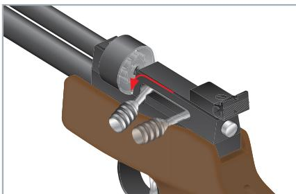
9. Close and lock the bolt by pushing the bolt handle forward and down.
