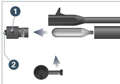
1. Open the CO<sub>2</sub> compartment as shown. If the CO<sub>2</sub> compartment cap 1 cannot be loosened by hand, use the screwed-in strengthening rod 2 to open the cap.
