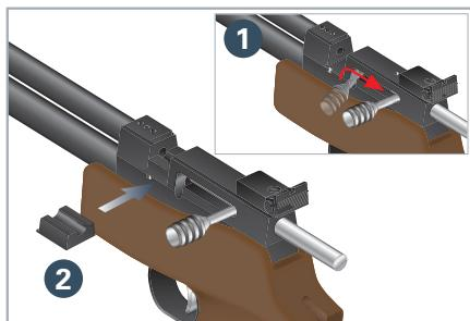
1. Pull the bolt handle backward to its open position **1** until a click sound is heard. Now insert the loading base **2**.
