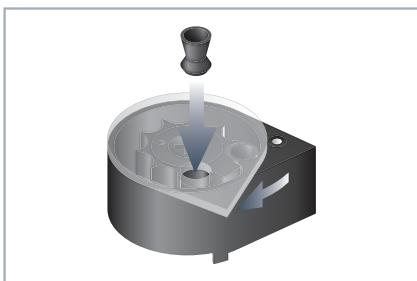
6. Turn the transparent plate clockwise to the next chamber and insert the next pellet.
