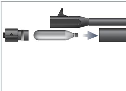
2. Insert a CO<sub>2</sub> capsule and close the CO<sub>2</sub> compartment with the CO<sub>2</sub> compartment cap. Tighten the cap quickly to avoid unnecessary gas loss.
