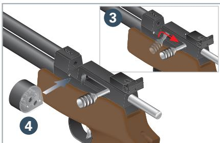
8. Pull the bolt handle backward to its open position **3** until a click sound is heard. Now insert the loaded magazine as shown **4**.
