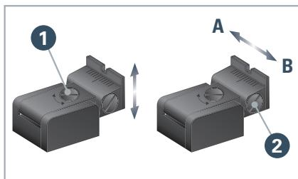
**Elevation adjustment:** If the point of impact is too high: turn screw **1** clockwise. If the point of impact is too low: adjust screw **1** counterclockwise.
