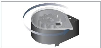
2. Rotate the transparent plate counterclockwise until it stops.
