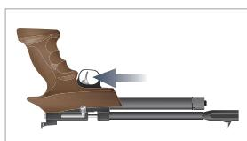
Clean your airgun at regular intervals (500 shots) using a CO<sub>2</sub> maintenance capsule. Remove all pellets from the airgun, insert the CO<sub>2</sub> maintenance capsule and close the CO<sub>2</sub> compartment. Hold the airgun as shown and fire at a safe target until the capsule is empty.
