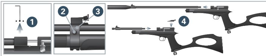
1. Using a hexagon (Allen) key, loosen the three barrel fastening screws **1**. Loosen the screw **2** of the barrel band **3** and remove the band. In the next step, pull out the barrel of the rifle (as shown in the figure)
