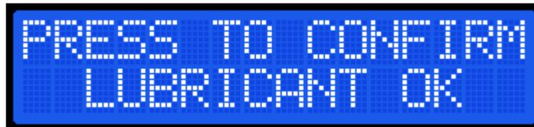
Press the rotary control knob to confirm the lubricant check. After this, the display will show the first page of the main menu; the target pressure display.
