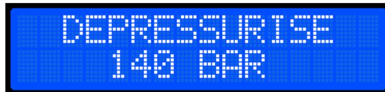
**DO NOT depressurise the system using any other method such as unscrewing the cylinder or using additional bleed screws located at the cylinder.**
