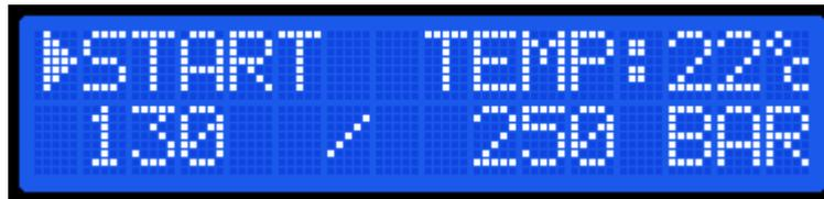
If no high pressure is detected in the system, only the target pressure will be displayed.
