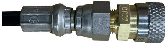
**Hill recommends using only fill probes and adaptors which are designed to allow the vessels' integrated non-return valve to close. This allows the moisture collected by the water separator to be drained via the bleed screw on the compressor.**
