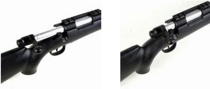
Hold the bolt handle continue to pull back until it locks in place. Do not lower the bolt handle. Push the bolt handle forward and lower to its original position and it is ready to fire.
