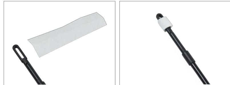
Cut the cloth or paper towel in the size as shown above. Fold the material to fit through the loop. Adjust the length of the material to smoothly enter the barrel. Otherwise too much material will get jammed in the inner barrel and can cause the hop up bucking to get out of place.
