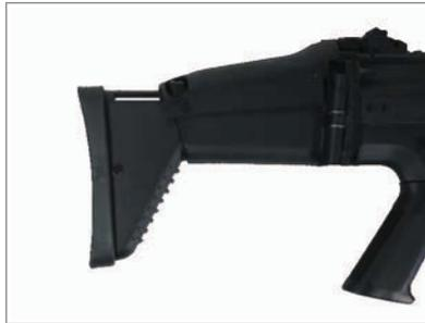
**Step 1.** Gently push the stock pin to the side. The stock pin is held in the stock by a small metal clip. With too much force applied to the stock pin the clip will become disconnected. Do not lose the stock pin and clip.
