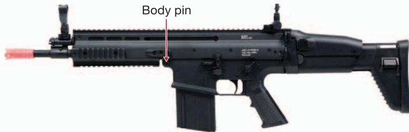
To drop the lower receiver press the body pin to the side. The body pin is held in the lower by a metal clip. Once the body pin is loose you are able to pivot from the rear and separate the lower. Make sure the bolt and charging handle is forward for an easier procedure.
