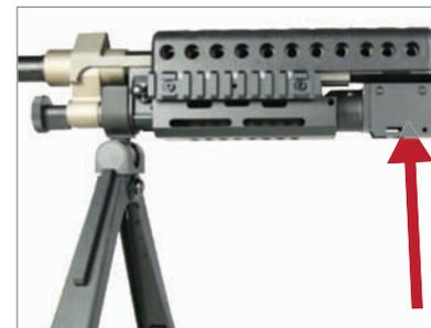
**Bipod 3.** Extend the bipod legs out and allow gun to rest. Press the bipod lock plate up to secure.
