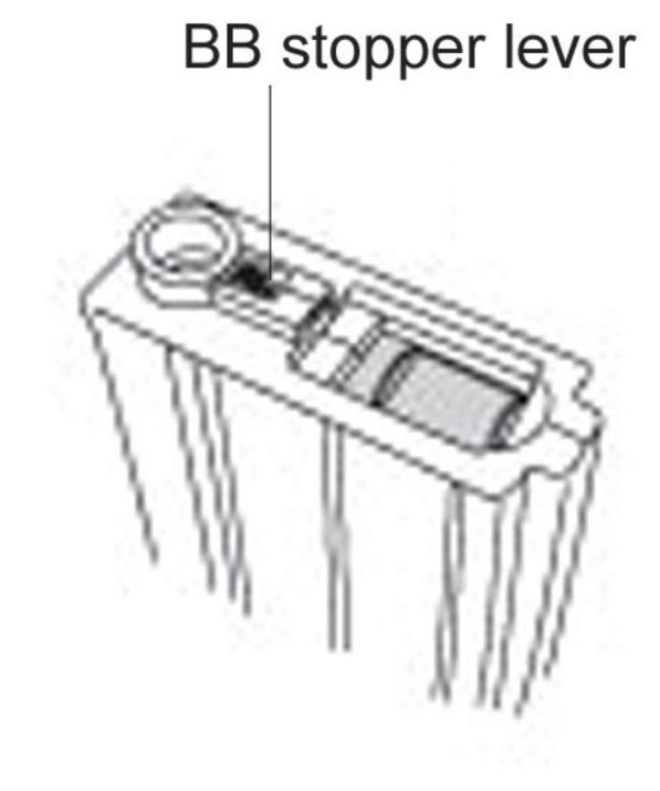
For storage release the remaining BB's to ensure correct operation next time, by pulling gently back on the BB stopper lever.
