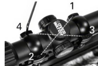
**CAUTION! DO NOT OVER-TIGHTEN THE SCOPE RING SCREWS. OVER TIGHTENING THE SCOPE RING SCREWS CAN CAUSE DAMAGE TO THE SCOPE OR RINGS, EFFECTING PERFORMANCE OR RENDERING IT INOPERABLE. THE GAPS BETWEEN THE TOP AND BOTTOM RING HALVES SHOULD BE EVEN ON THE LEFT AND RIGHT SIDE OF BOTH SCOPE RINGS.**
