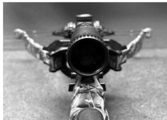
**Note:** During step 3, the scope rings may need to be re-positioned on the scope mount if you run out of eye relief adjustment.
