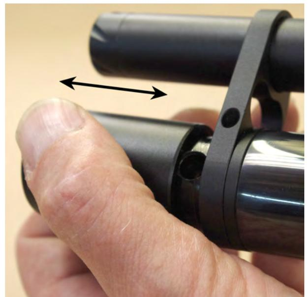
Once the required fill pressure has been reached (see chart below for filling pressure information) close the valve or stop pumping. Vent the system using the vent screw (see arrow below) on your filling kit and withdraw the probe from the filling valve body. If the probe does not slide out with ease, check to make sure the hose is completely empty of air by opening the vent screw again.
