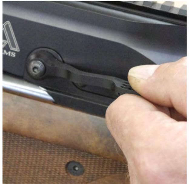
***Close the lever to its starting position to lock the lever ready to fire.***
