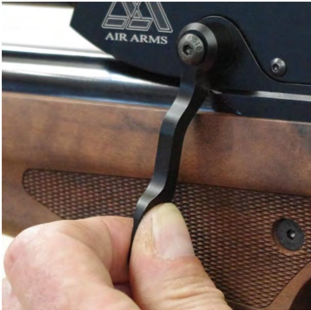
***Push the cocking lever forwards to the end of its travel. The rifle indexes and sets the trigger unit.***
