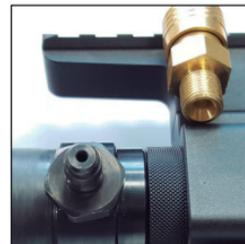
To fill your rifle, attach the adapter to the hose of your fill device and then attach it to the gun's fill port.
