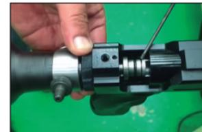
Fasten set screw and re-install top rail.
