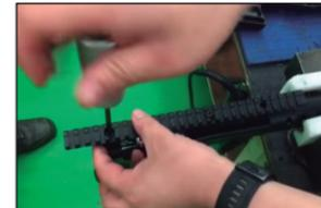
Install the cylinder keeping a 0.5mm-1mm gap between barrel and valve.
