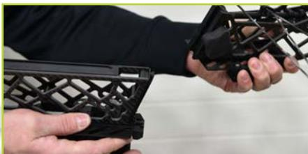
Line up the female dovetail on the head with the male dovetail on the main frame. Slide the two together until the spring pin snaps into place.
