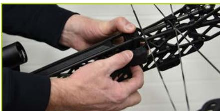
To take apart, loosen the same thumb knob, pull back on the rubber lever of the spring pin and slide apart.
