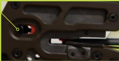
The safety/fire switch has a black post that is visible from either side of the trigger box.
