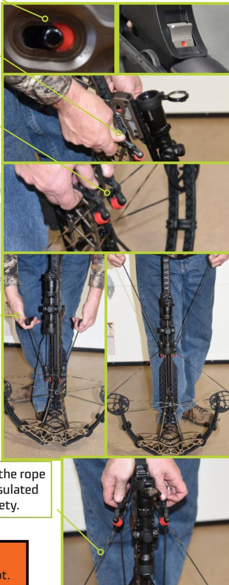
Slowly let up on the handles and remove the rope cocker. The crossbow string is now encapsulated in the trigger box and the trigger is on safety.
