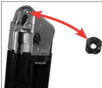
If the rubber lip on the valve is worn, the gun might shoot two BBs at once. To remedy this, remove the rubber lip and use a little instant glue to affix the spare part supplied.
