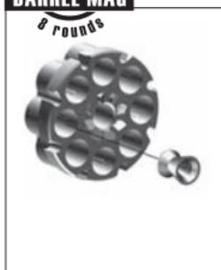
Load pellets into cylinder magazine.
