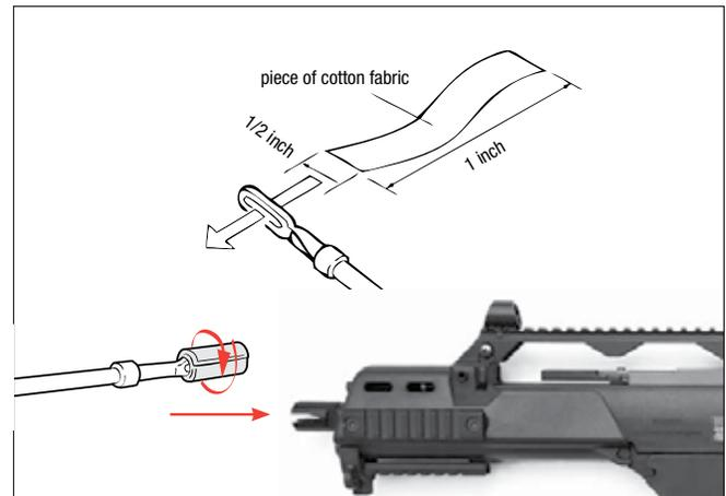
Put the safety ON SAFE and remove the magazine. Prepare a thin rod with a length of approx. 16 inches. Attach a piece of cotton fabric to its end and clean the barrel with some silicone oil.
