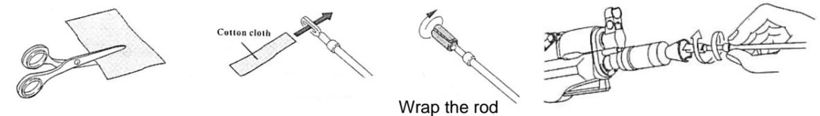
Maintenance is needed when bullet speed becomes slow. Wrap a cotton cloth on the rod. Hold the leading end of the rod and insert rod into the barrel while turning the rod to clean the barrel inside
