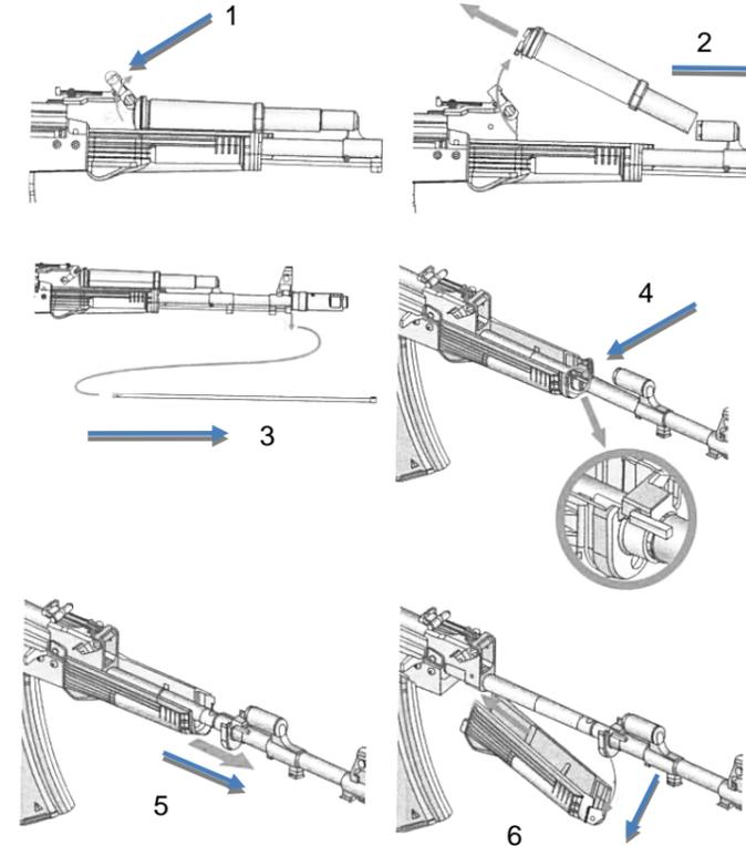
1. Push the upper hand guard fixer upwards
