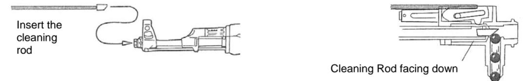
1. Make sure to insert the cleaning rod AFTER returning the hop up lever to NORMAL position. (HOP OFF)
