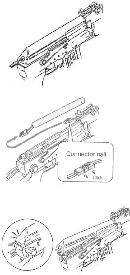
1) Remove the receiver top from its rear while pressing the receiver top catch button
