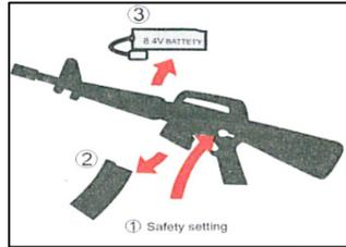
Remove magazine and battery during storage. Set the fire selector to safe when unused
