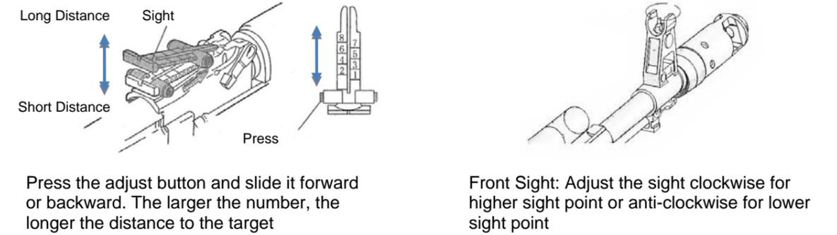
Press the adjust button and slide it forward or backward. The larger the number, the longer the distance to the target
