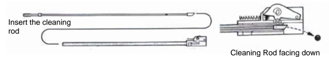
1. Make sure to insert the cleaning rod AFTER returning the hop up lever to NORMAL position. (HOP OFF)
