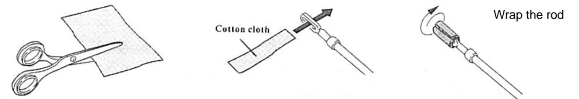
Maintenance is needed when bullet speed becomes slow. Wrap a cotton cloth on the rod. Hold the leading end of the rod and insert rod into the barrel while turning the rod to clean the barrel inside
