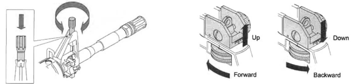
Use Calibrating tools to adjust the sight. Turning anti-clockwise to lowers the bullet hitting point or clockwise to higher the bullet hitting points
