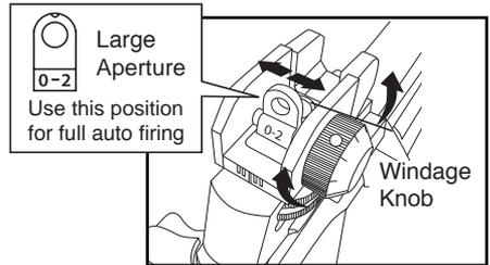
The sight assembly is marked in millimeters for precise adjustments
