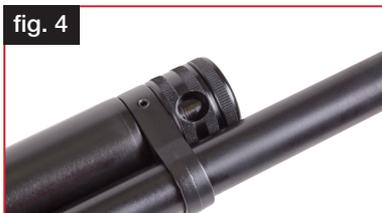
2) When charging is complete, bleed the excess air using the fill apparatus bleed screw and remove the fill adapter from the rifle. When finished, rotate the protective cover to prevent contamination of the fill port (fig. 4).
