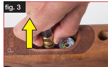
2) When charging is complete, bleed the excess air using the fill apparatus bleed screw. Once the line is bled, pull back on the fill adapter collar and remove the fill adapter from the rifle (fig. 3).
