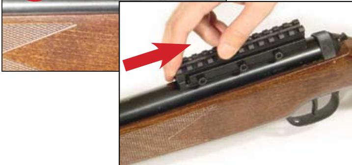
**3** Hold the mount base in front of the dovetail. Align the rear of the mount base with the front end of the dovetail rail. Slide the mount base backward on the dovetail rail until the recoil stop shoulder of the mount base contacts the front end of the dovetail rail.
