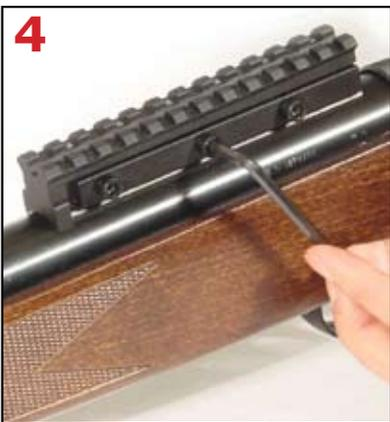
**4** Tighten the 3 side-locking screws to firmly lock the mount base. Make sure you don't over-tighten them.
