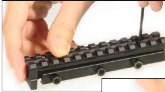
**2** Use the correct included Allen wrenches to loosen the 3 side-locking screws & the stop-pin in the mount base.
