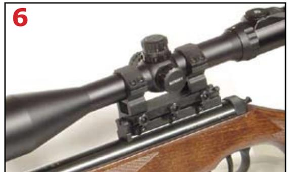
**6** The mount base is now available for mounting a scope and either 1-piece or 2-piece mounts.
