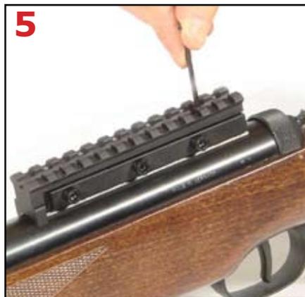
**5** Properly tighten the stop-pin from the top of the mount base.
