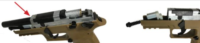
Press barrel release button to remove barrel. The recoil spring guide rod assembly will now be free to remove. With .177 rod or similar size object, push jammed pellets through barrel and out the muzzle end.
