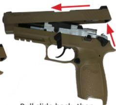
Pull slide back, then up and forward to remove.
