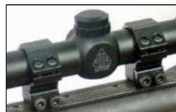
1. Turn the Hex Screws counterclockwise with the included Allen wrench to widen the locking plate and provide the needed mounting clearance to evenly seat onto the Dovetail Rail.
