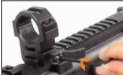
3. Should the QD mount base be loose, unlock the Cam Lever and use the included Allen Wrench to adjust the Hex Screw found within the Cam Lever Housing. Turning the Hex Screw clockwise will increase the locking plate tension by decreasing the clamping width.
