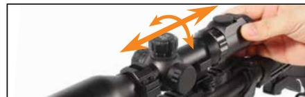
2. Place the scope within the scope ring bases, taking care to properly adjust for a comfortable eye relief and that the scope's reticle is leveled.
