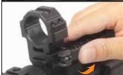
4. Should the Cam Lever not fully turn into the locked position and you feel heavy resistance, the locking plate tension is too high. Use the included Allen wrench to adjust the Hex Screw counterclockwise to decrease the locking plate tension by increasing the clamping width.
