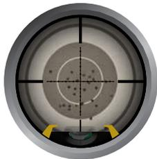
3. The purpose of the internal bubble leveler is to ensure a consistent orientation of the scope during each shot. When optimum accuracy and confidence is a must, you do not want the scope tilted to the left or right of center when taking that critical shot. The scope must have been installed correctly positioned and leveled with the specific application being used in the beginning.
