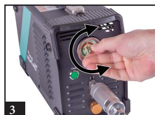
**! WARNING** DO NOT OVERFILL AIR CYLINDERS OR AIR GUN TANKS, AS THIS CAN CAUSE SERIOUS INJURY OR DEATH. NEVER SET THE OUTPUT PRESSURE/AUTO SHUT OFF ABOVE 4500 PSI (310 BAR).
