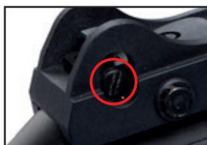
To adjust the windage, turn the screw clockwise to move the point of aim to the right.
