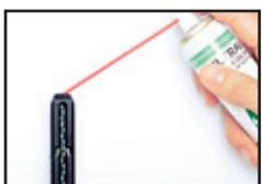
Add a few drops of silicone oil on the BB located in the BB loading hole. Reinsert the magazine into the Airsoft gun.
