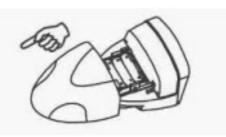
3.2.3 Insert 6 new batteries into the BATTERY COMPARTMENT. Cares should be taken for the polarities symbols (+ and -) which are marked on the connection terminals of the detector and the batteries. The polarities of the battery must be matched with the polarities of the terminals.
