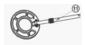
3.1.2 Slide the UPPER STEM (12) towards the SEARCH COIL (14) as indicated by an arrow until you can see a micro-plug metal connector. Pull out the plug so that you can hold it on your hand.
