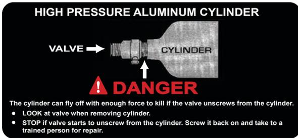
Look for a rotation indication mark between tank and bottle. Ensure line matches between two pieces. IF THE LINE DOES NOT MATCH DO NOT FILL THE CYLINDER.
