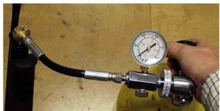
hose, if you do not vent the hose you will not be able to remove the female from the rifle). Now the female connector can be removed from the rifle and end cap (S483) can be replaced over the male connector ensuring not to over-tighten.
