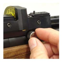
On the left hand side of the rifle is a indicator to help select your most common power settings += High. -= Low. The marks do not indicate a particular power as this would change depending on the pellets used.
