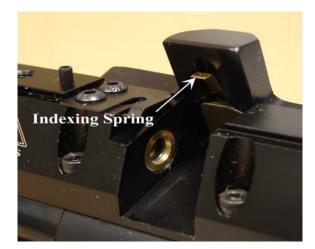
Be very careful not to damage the Indexing spring when demounting or mounting the magazine. Follow the instructions carefully.
