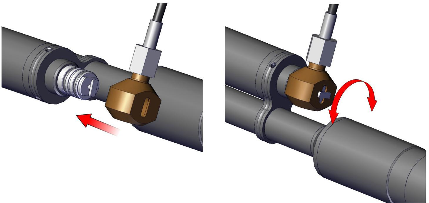
With the female locked onto the male the rifle can be filled.
