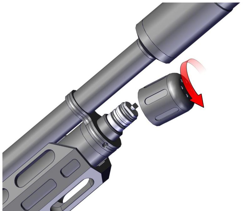
Push the female connector over the male, ensuring the Tee piece of the male connector fits through the slot on the female. Once the Tee piece is through the slot, twist the female to lock onto the male.
