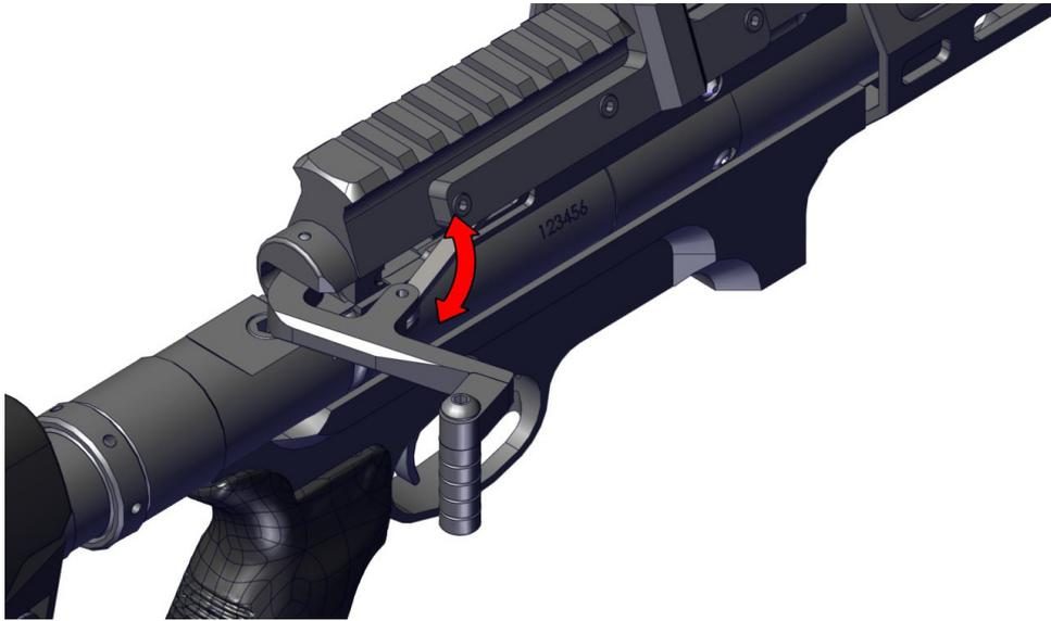
To refit the magazine simply slide it back into the action until it is fully home. Ensure the cocking lever is in the rear position the whole time. Once the magazine is fitted the lever can be closed.
