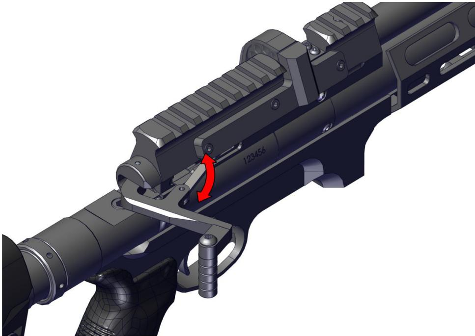
Note: It is very important that the cocking lever is pulled back to the correct position in one positive motion. The magazine indexes to the next pellet position as the bolt is retracted and it is possible for a partial index if the lever is not pulled back fully.
