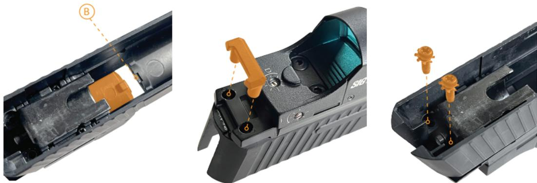
Place the SIG Air Reflex Sight and Airgun Optics Plate assembly onto the slide and ensure that the plate seats into the notch **(B)** under the front of the sight plate opening. Replace the rear sight with the included optics plate anchor to allow proper clearance to access the reflex sight locking screws.
