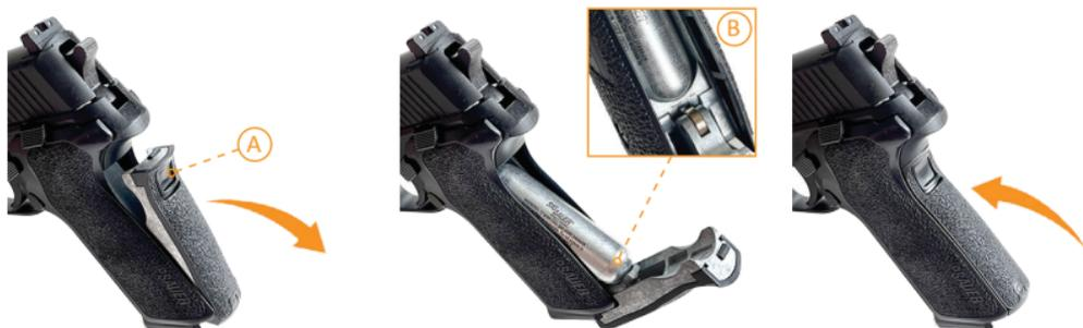
Pull down on the latch (A) and swing the backstrap of the grip open. Insert the CO2 cartridge into the grip nose first and ensure that the bottom of the cartridge is fully seated into the cup (B) of the loading mechanism. Closing and latching the backstrap will pierce the CO2 cartridge and pressurize the air gun for operation. See section 11.0 for instructions on depressurizing the air gun.
