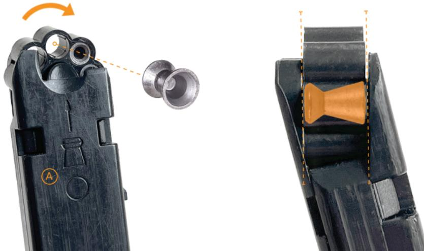
Insert pellets or steel BBs into the chamber of the rotary clip located at each end of the magazine and then rotate the clip clockwise until all chambers are loaded. When loading pellets, ensure the pellet is inserted nose first from the back of the magazine indicated by the ammunition marking (A). The pellet must be fully seated into the chamber so that it is flush with the rear of the rotary clip and does not extend past the front.
