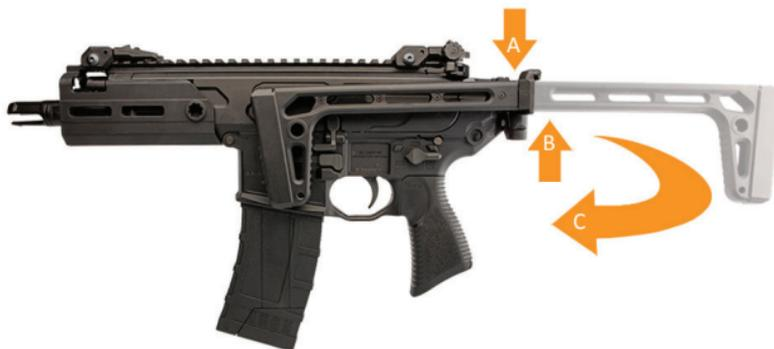
The stock can be folded by grasping the stock near the hinge and, while pressing against the top of the hinge **(A)**, squeeze the stock upwards towards the hinge to unlock it **(B)**. While doing so, pivot the stock to the left to fold it against the receiver **(C)**. To unfold the stock, pivot the stock away from the receiver until it locks in the extended position.
