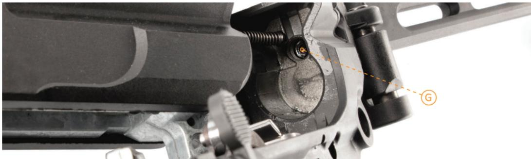
**Reinstalling Upper:** Align the recoil spring guide with the receptacle **(G)** in the back of the upper receiver and then slowly allow the rear lug of upper receiver to seat down into the lower receiver. Pivot the front of the upper receiver down so that the front lug aligns with the lower receiver. Once the pivot and takedown pin holes are aligned, push the pins back through the receiver until fully seated. Cycle the charging handle to ensure the bolt functions properly after reassembly.
