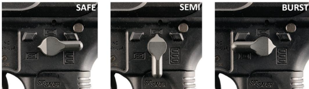
Either the left or right selector switch can be used to change the fire mode of the airgun. In **SAFE**, the trigger will be physically locked to prevent accidental firing. In **SEMI**, the airgun will fire one (1) BB for each pull of the trigger. In **BURST**, the airgun will fire three (3) BB's for each pull of the trigger.
