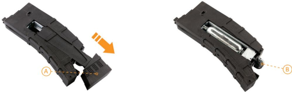
Press the magazine release button to remove the magazine from the airgun. Pull down on the bottom rear corner of the magazine **(A)** to remove the cover. Loosen the screw on the bottom of the magazine **(B)** before inserting the 12g CO2 cartridge into the cavity as shown. Then, tighten the screw on the bottom of the magazine. The sound of gas escaping will be heard as the seal is pierced. Continue tightening the screw until snug, then give one final 1/4 turn.
