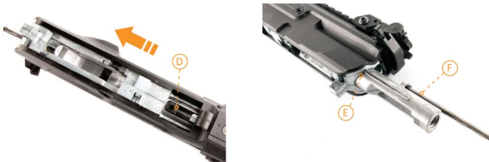
**Removing Bolt:** Press rearward on the loading nozzle **(D)** to separate it from the chamber and begin pushing the bolt from the upper receiver. Once the end of the bolt reaches the rear of the upper receiver, the bolt can be grabbed from the rear and pulled completely from the upper receiver.
