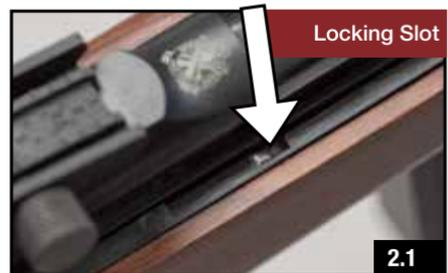
Once the pin is in the slot, the bolt will be held in the open position (Fig. 2.2). To release the bolt, pull back on the charging handle slightly and release it.
