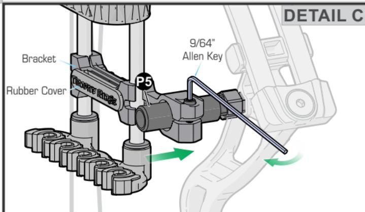
**STEP 4** Attach the bottom assembly to the lower post. See Figure 2 & Detail D.
