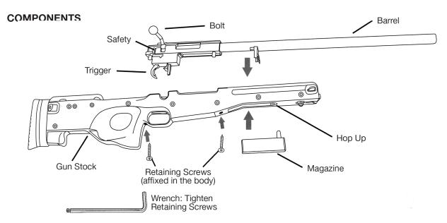
**1** SAFETY SETTING (Always set the safety lever to safe position before firing)
