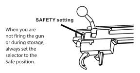
When the safety lever is set to the "On" position, the trigger will not move. Please do not pull the trigger, otherwise you may damage the gun.
