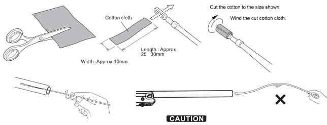
Hold at the leading end of the rod and insert the rod into the barrel while turning the rod.
